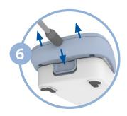
Press battery latch down and slide charger off battery.
