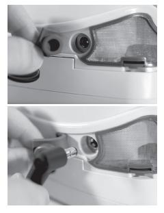
2. Connect the AC power cord to the AC power brick.
