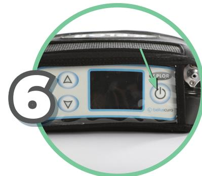
6 Turn on the X-PLO<sub>2</sub>R by pressing the power button for 2 seconds. Set the flow setting to your prescribed setting and use normally.
