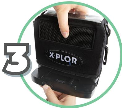
Remove the battery from the X-PLO<sub>2</sub>R.
