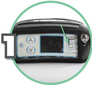
Turn off the X-PLO<sub>2</sub>R™ by pressing the power button for 2 seconds.
